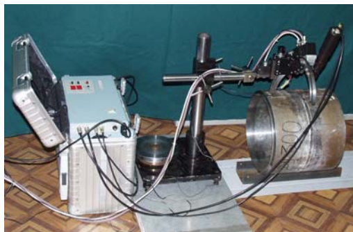
Measuring tube fragment made of steel 12X18H10T
